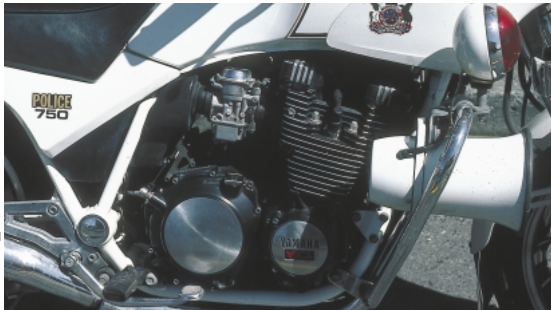
Figure 5.19 An air-cooled engine has no radiator. How do the fins on this engine keep it from overheating?
