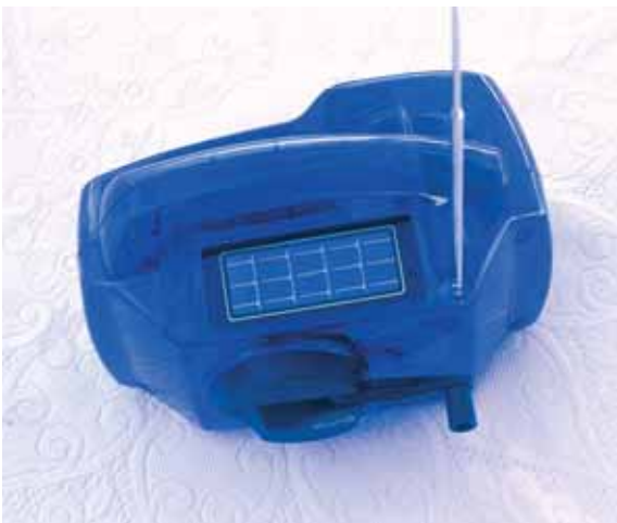
Figure 7.27 Recently, solar-powered and hand-wound radios were developed for use in countries where electricity is scarce. Many Canadians now use these radios because they do not need batteries or an electricity source.
