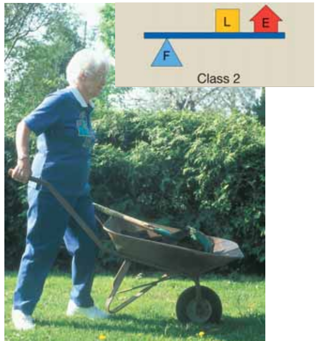
Figure 7.15 A wheelbarrow is a second class lever. Note the location of the fulcrum, effort, and load.
