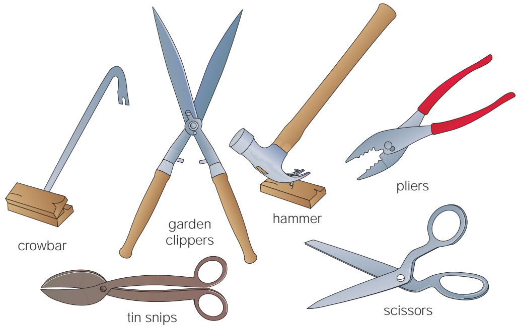
Figure 7.14 Many common household tools are examples of the first class lever. Identify the fulcrum, load, and effort for each.
