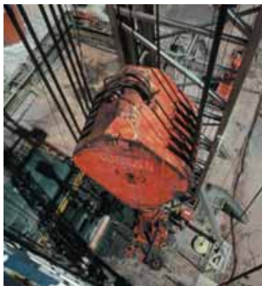
Some oil rigs move loads with pulleys like the one you used in Part 3. This is called a moveable pulley because the pulley moves with the load.
