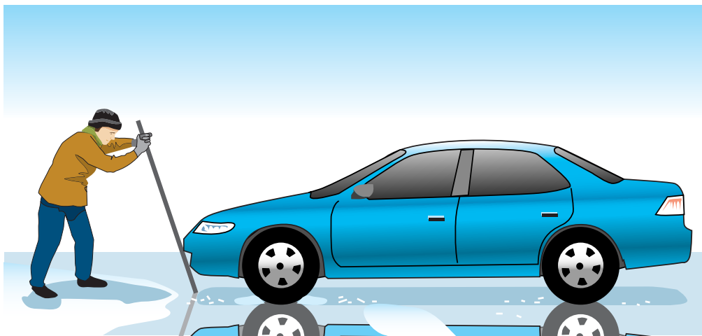
Figure 7.18 When the load distance is small, a large load can be moved with little effort. But don't try this if you have a plastic bumper!
