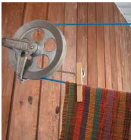
Clotheslines have pulleys like the one you used in Part 1. This is called a fixed pulley because the pulley does not move with the load.
