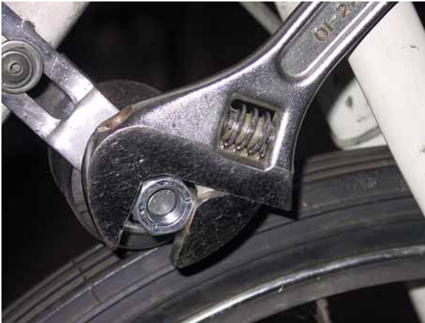
Figure 7.21 Both the wrench and the nut will turn through 360^\circ . By the time the wrench has gone completely around, it has acted like a large wheel. This large wheel is easy to turn compared to the smaller wheel, the nut. A little effort on the wrench moves a heavy load on the rusty nut.
