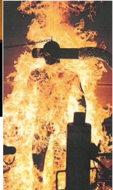
Figure 6.14 Harry is a mannequin at the University of Alberta. His 110 sensors measure the rate and the amount of heat transfer from fires.
